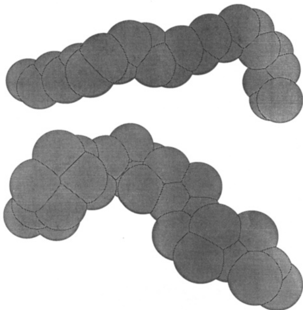
Figure 6. Space-filling views of PIB (lower) and PE (upper) chains generated by assigning van der Waals radii = \sigma/2 of Table II to the groups.
